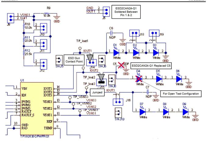
Figure 1-3. TPS92630EVM Schematic With Protection and Testing Modifications
