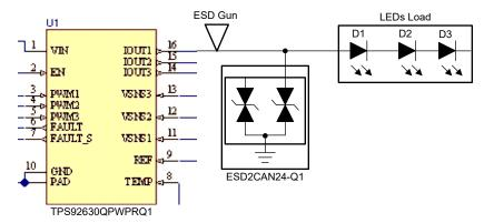
Figure 1-1. Loaded Test Configuration
