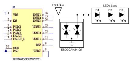
Figure 1-2. Open Test Configuration
