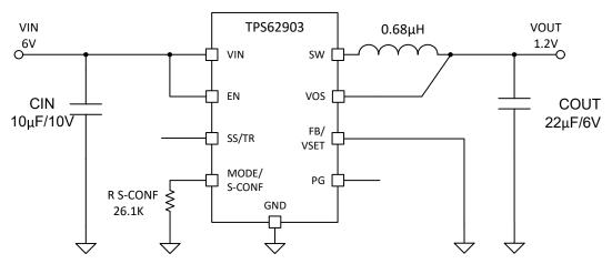
Figure 1-1. Design Example Schematic
