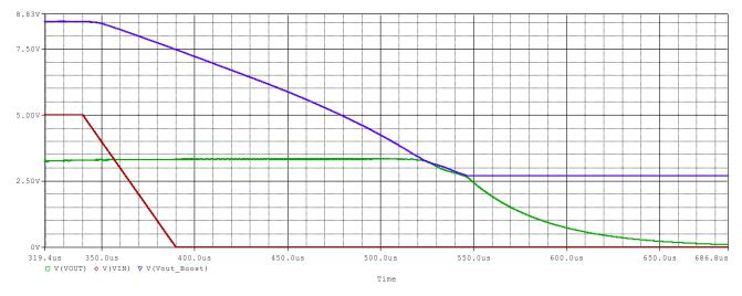
Figure 3-2. PSpice Simulation Results (VIN, VBOOST.OUT, VOUT)
