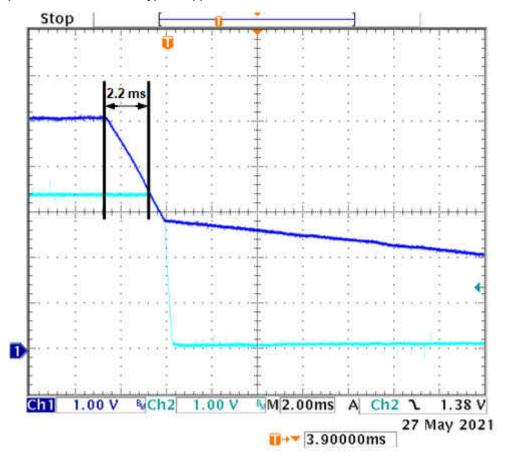
Figure 3-3. Test Waveform With the Typical Application TPS62130 Method
