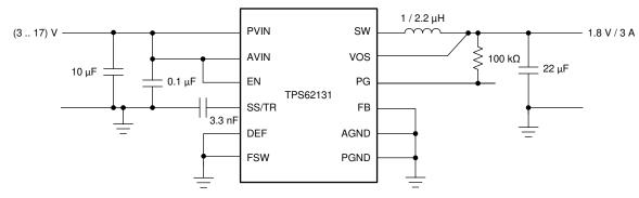
Figure 1-1. Typical TPS62130 Application Circuit
