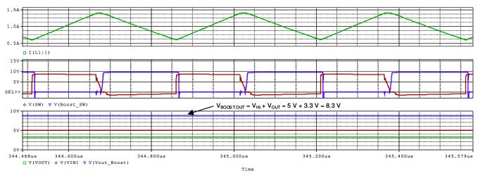
Figure 3-1. PSpice Simulation Results in Steady State
