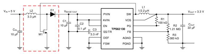
Figure 2-1. Proposed Application Circuit Using Boost Pre-Regulator
