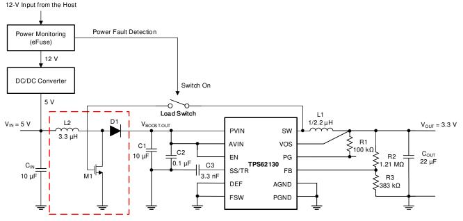
Figure 2-2. Application Example With Load Switch
