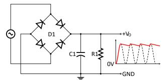
Figure 1. Classic Full-Wave Diode Bridge DC Rectifier
