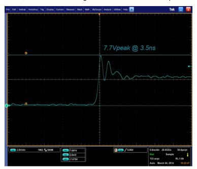
Figure 5-2. Added RC Snubber (3.3 ohm + 470pF) on PH node
