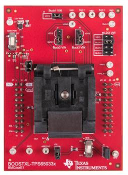
Figure 1. TPS650330-Q1 Programming BoosterPack™ EVM
