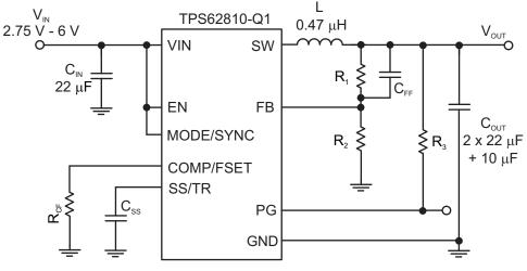
Figure 1. Typical TPS6282X Application Circuit
