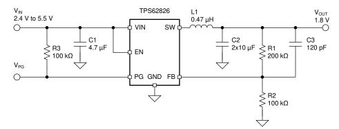
Figure 4. Typical TPS6281X Application Circuit
