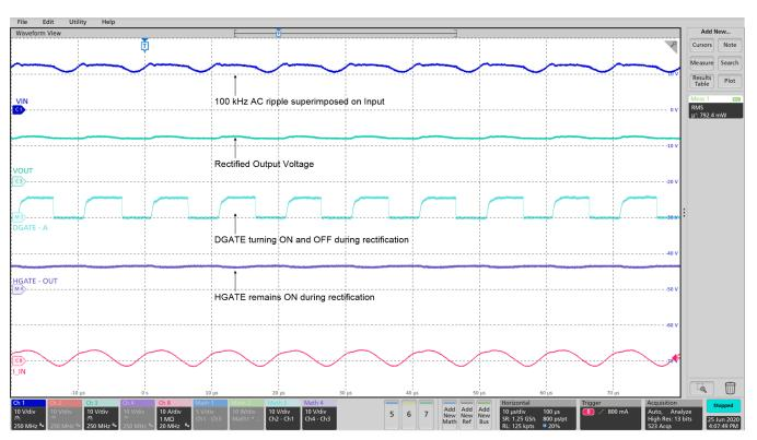
Figure 8. LM7481-Q1 Active Rectification at 100 kHz - BUK9J2R8-40H
