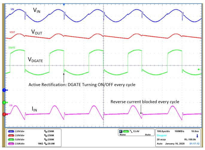
Figure 5. LM7480-Q1 - Active Rectification of 2-V Peak-Peak 5 kHz AC Ripple
