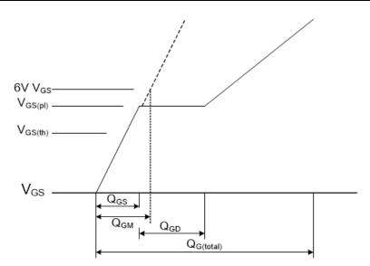
Figure 7. Gate Charge Derating for Active Rectification
