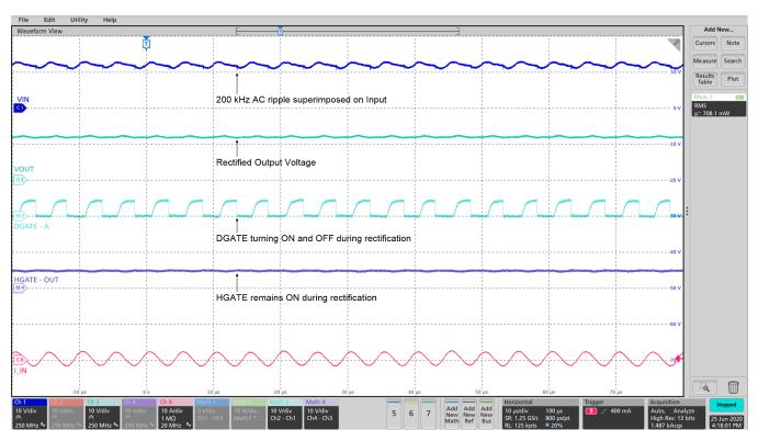
Figure 9. LM7481-Q1 Active Rectification at 200 kHz – BUK7Y3R5-40H
