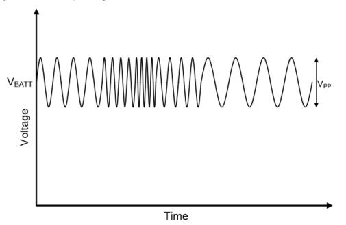
Figure 1. AC Super Imposed Test
