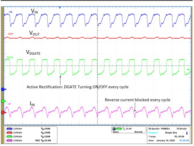
Figure 6. LM7480-Q1 - Active Rectification of 2-V Peak-Peak 30-kHz AC Ripple
