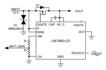
Figure 4. Simplified Schematic of Ideal Diode Controller LM7480-Q1
