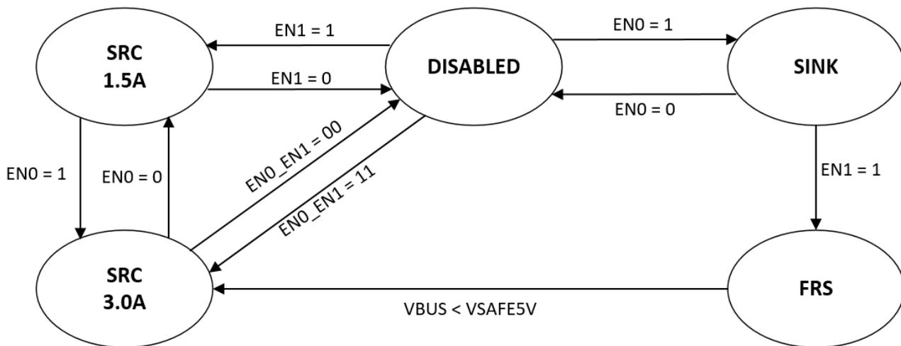
**Figure 7. Sink and Source With FRS State Machine**
