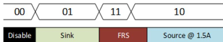
**Figure 8. Sink to 1.5-A Source FRS Transition**
