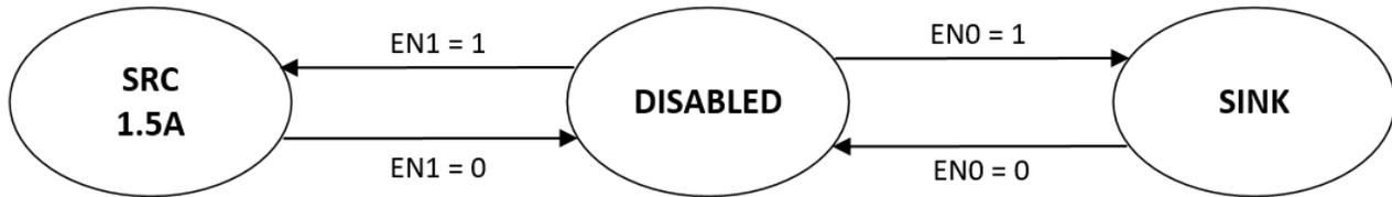
Figure 3. Sink With 1.5-A Source State Machine
