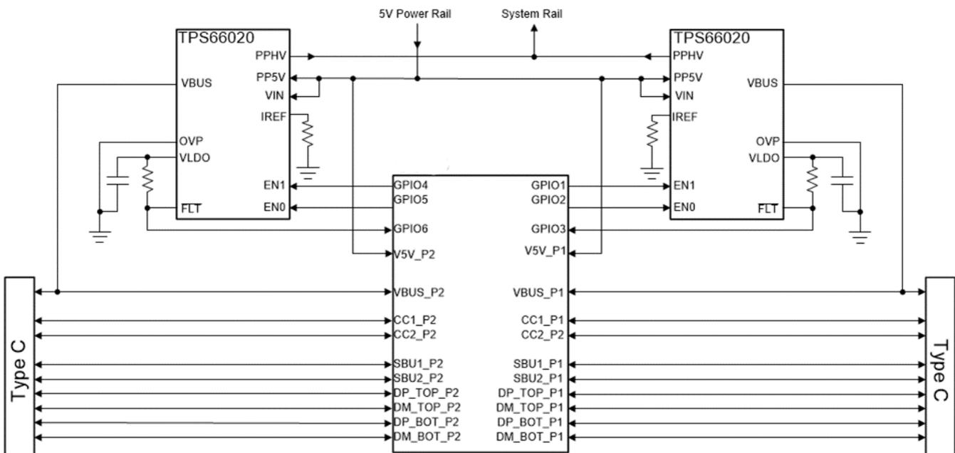
**Figure 1. Typical Two Port System With TPS66020**
