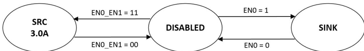
Figure 5. Sink With 3.0-A Source State Machine
