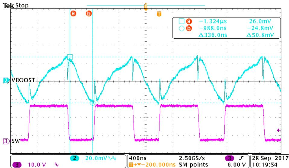
**Figure 9. BOOST Ripple Under  $V_{LNB} = 18.2$  V, Load = 1-A Condition**
