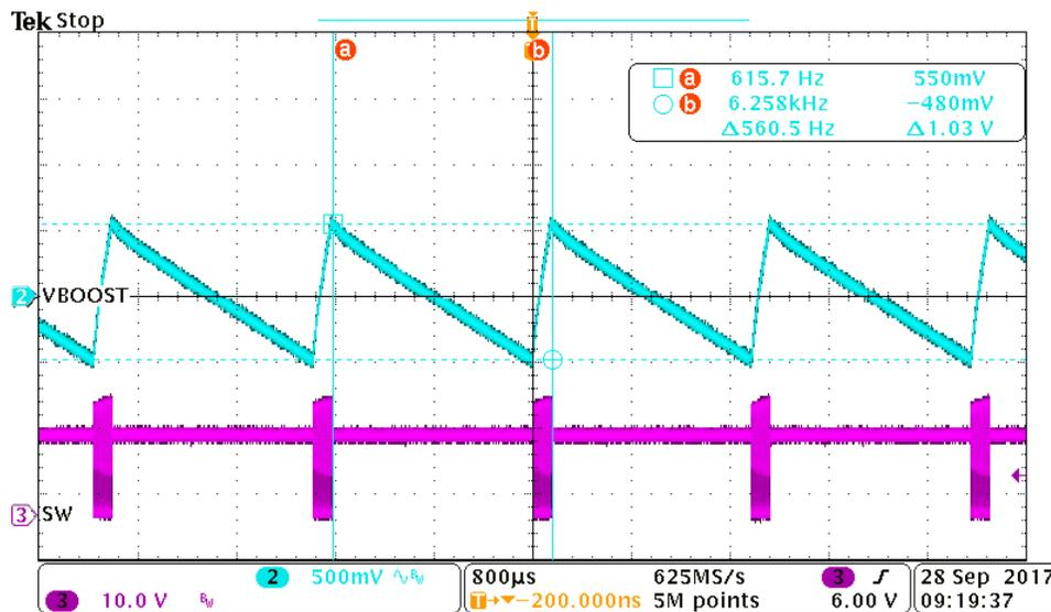
Figure 1. BOOST Ripple Amplitude and Frequency in TPS65235
