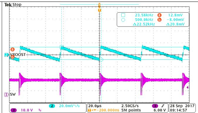
Figure 6. TPS65235-1:  $V_{PP}=20.8$  mV,  $F_{RIPPLE}=22.5$  kHz
