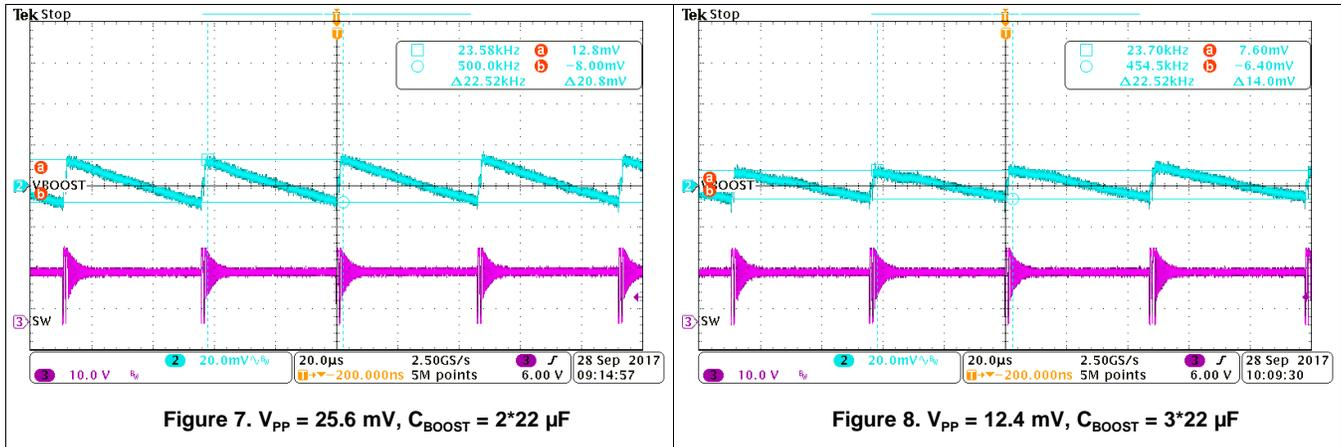
When selecting the MLCC as BOOST output filter capacitor, the capacitance derating should be considered. The following introduces a method to evaluate the MLCC actual capacitance.
