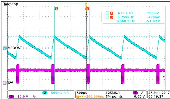
Figure 5. TPS65235:  $V_{PP}=1.03$  V,  $F_{RIPPLE}=560.5$  Hz
