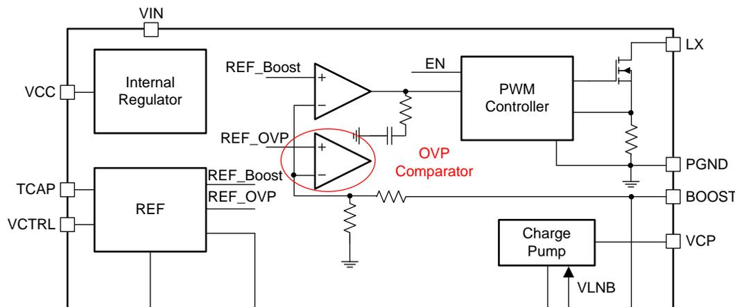
**Figure 4. OVP Comparator Block Diagram**
