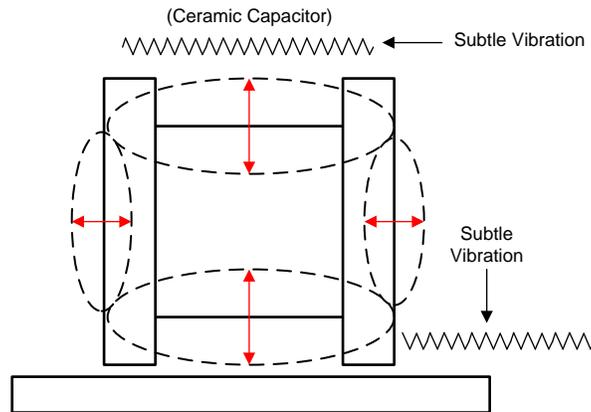
Figure 3. MLCC and PCB Subtle Vibration
