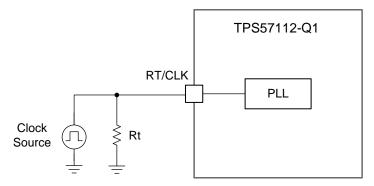
Figure 1. Synchronizing to a High-Impedance External Clock Source
