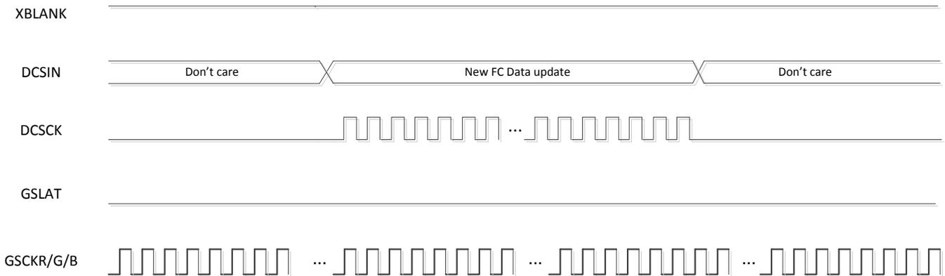
**Figure 4. New Data Update for Analog Dimming**
