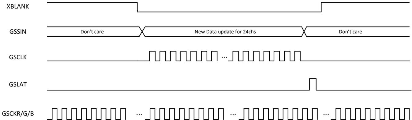
**Figure 3. New Data Update for PWM Dimming**
