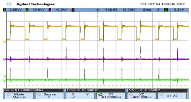
Figure 3. MSP430 Clock Output (Channel1) and Gate Drive for each MOSFET at No Load
