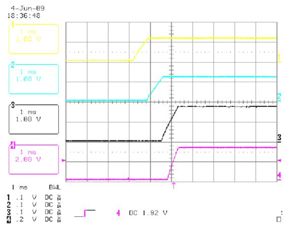
Figure 3. Shows Sequencing in Start-Up Waveform
