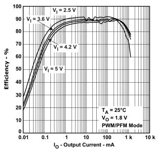
Figure 6. DCDC3: Efficiency vs Output Current
