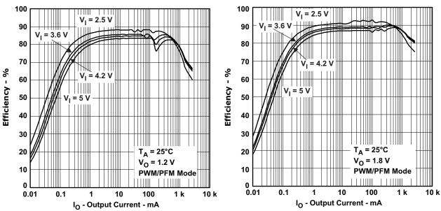
Figure 4. DCDC1: Efficiency vs Output Current
