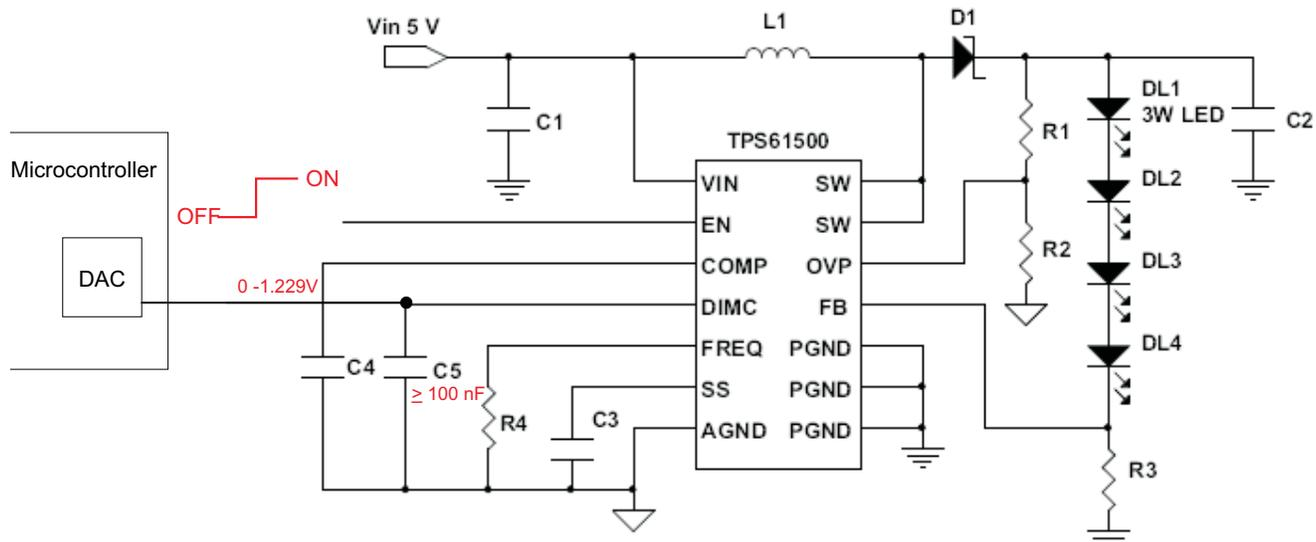
**Figure 1. Circuit for the TPS61500 to Perform Analog Dimming Using an Injected Analog Signal**
