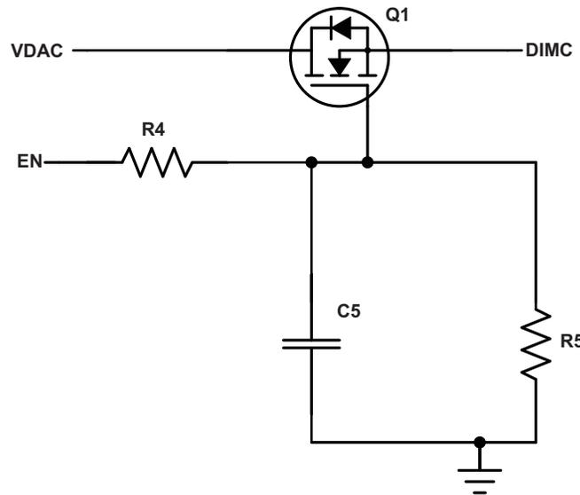
Figure 2. Isolation Circuit With RC Delayed Turnon
