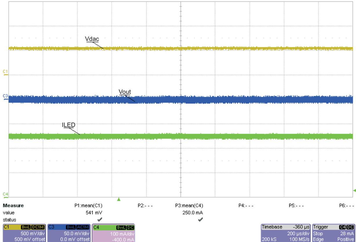
Figure 4. Output Voltage and LED Current With  $V_{IN} = 5 \text{ V}$  and  $V_{DAC} = 0.61 \text{ V}$
