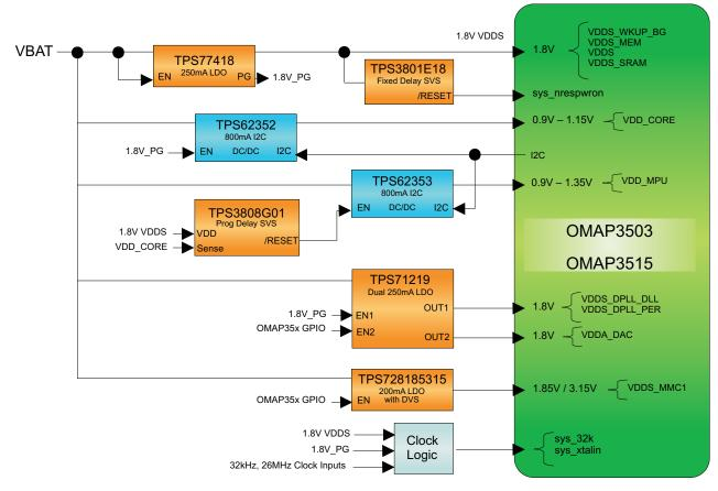
Figure 3. TPS6235x Power Solution Block Diagram
