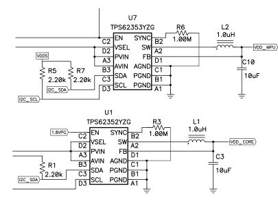
Figure 9. TPS6235x Circuitry to Power OMAP35x Core Voltages
