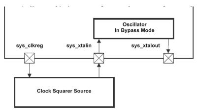
Figure 6. Clock Squarer Source Connection
