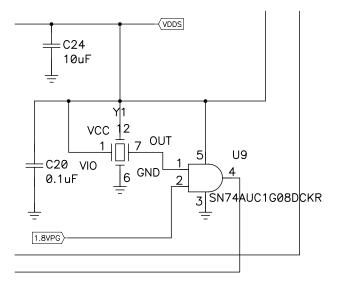
Figure 2. 32-kHz Clock Circuitry
