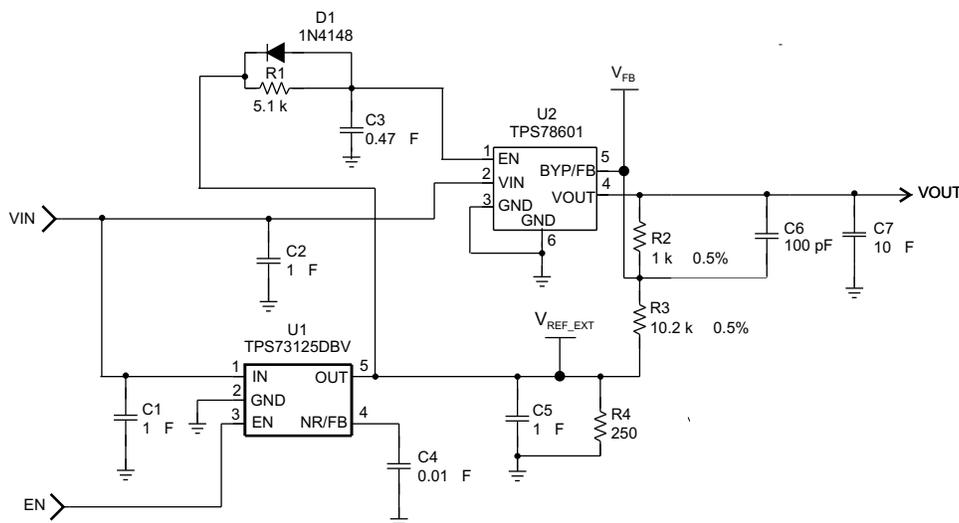
**Figure 3. TPS78601 Providing 1.1-V Output**
