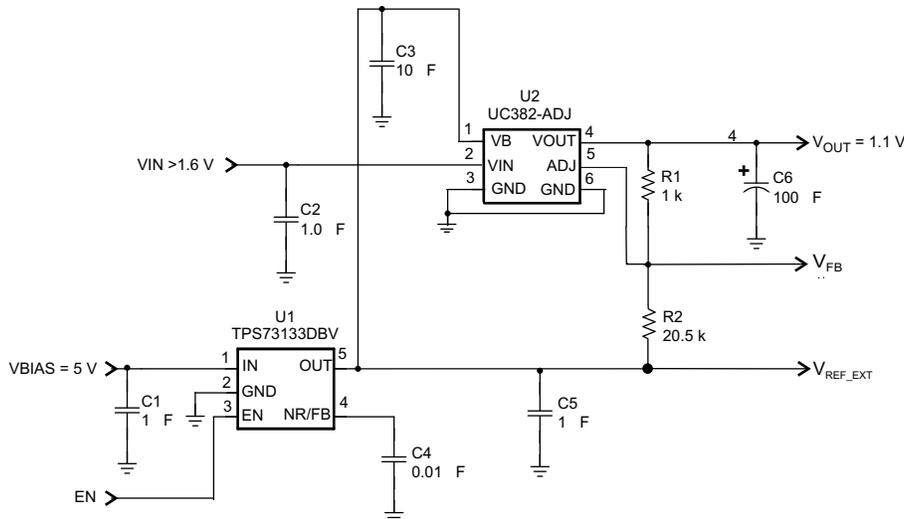
**Figure 2. UC382-ADJ Providing 1.1-V Output**
