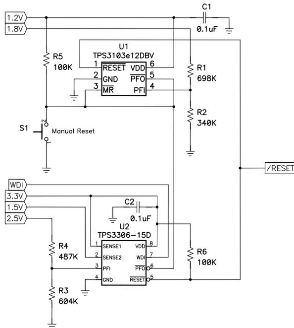
Figure 1. SVS Solution to Monitor Five Different Voltage Rails
