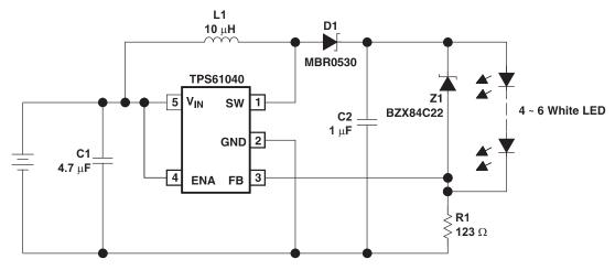
Figure 1. Constant Current LED Drive Supply
