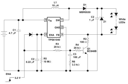
Figure 5. Modification to Reduce Turnon Delay
