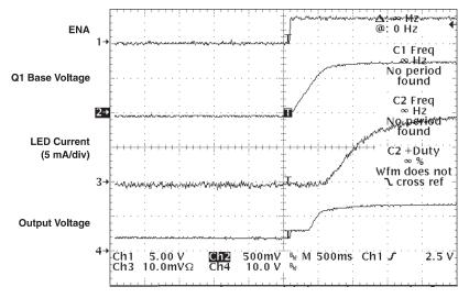
Figure 3. Waveform During Turnon
