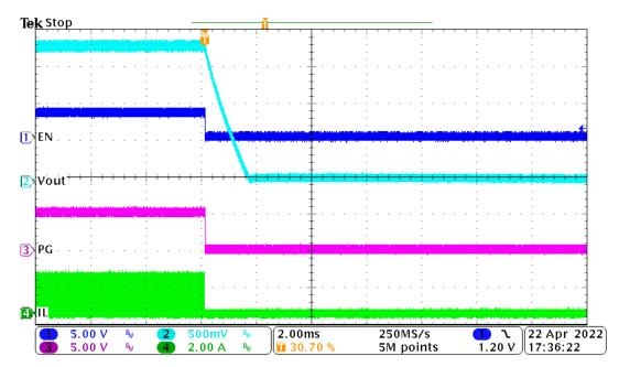
Figure 4-4. TPS51384EVM Shutdown Relative to EN, I<sub>OUT</sub> = 0.1 A
