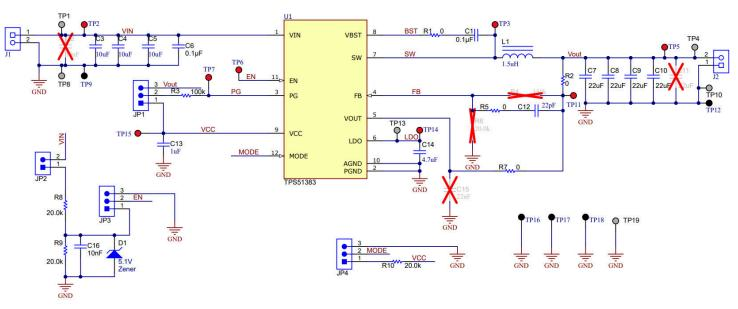
Figure 6-3. TPS51383EVM Schematic Diagram
