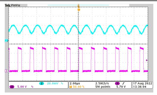
Figure 4-7. TPS51383EVM Output Voltage Ripple, I<sub>OUT</sub> = 8 A
