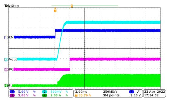
Figure 4-2. TPS51384EVM Start-Up Relative to EN, I<sub>OUT</sub> = 0.1 A
