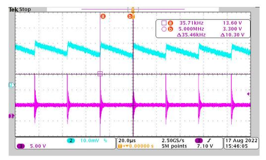
Figure 4-6. TPS51383EVM Output Voltage Ripple, I<sub>OUT</sub> = 10 mA, OOA Mode
