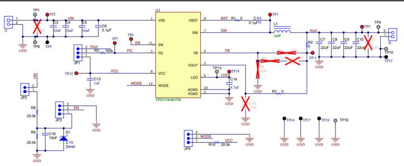
Figure 6-4. TPS51384EVM Schematic Diagram
