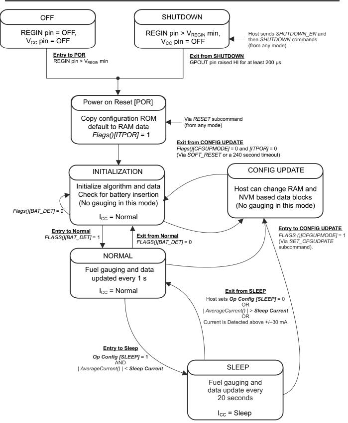
Figure 2-1. Power Mode Diagram
