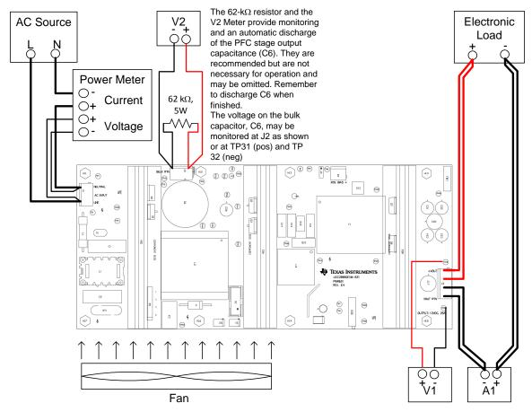
Figure 3. UCC29950EVM-631 Recommended Self Bias Test Set Up
