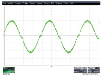
Figure 21. UCC29950EVM-631 Input Current (230-V<sub>AC</sub>, 50-Hz, full load 1 A/div.)
