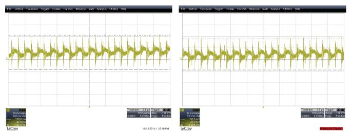
Figure 24. UCC29950EVM-631 Output Noise (115-V<sub>AC</sub>, 60-Hz input, full load)
