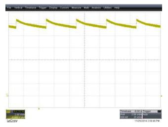
Figure 26.  $V_{OUT}$ , No Load, Aux Bias, Burst Interval is 340 ms,  $\Delta V_{OUT}$  is 400 mV
