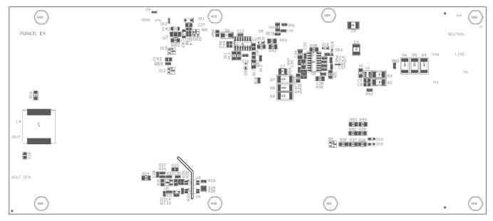
Figure 35. UCC29950EVM-631 Bottom Layer Assembly Drawing (bottom view)
