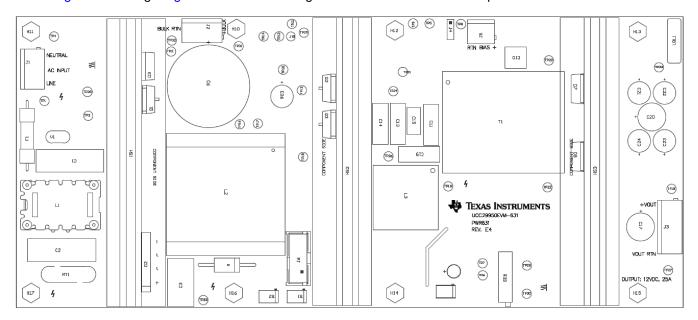
Figure 34. UCC29950EVM-631 Top Layer Assembly Drawing (top view)
