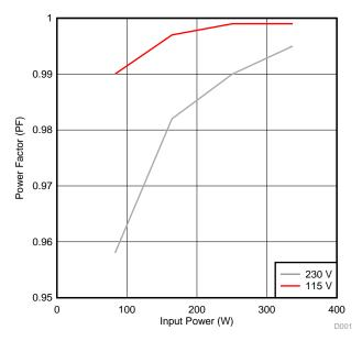
Figure 18. Power Factor vs Input Power
