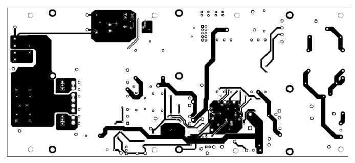
Figure 36. UCC29950EVM-631 Top Copper (top view)
