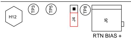
Figure 5. J4 Link Setting for Self Bias Mode
