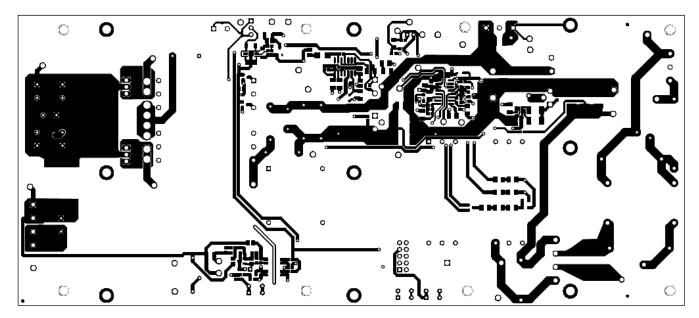
Figure 37. UCC29950EVM-631 Bottom Copper (bottom view)
