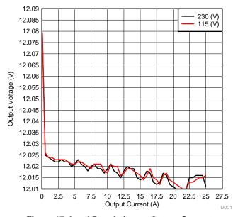
Figure 16. Line Regulation vs Input Voltage
