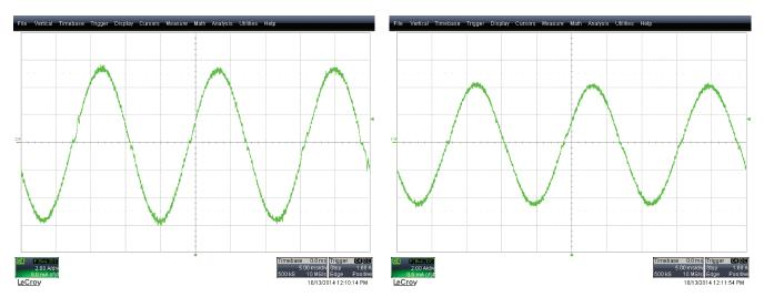
Figure 19. UCC29950EVM-631 Input current (90-V<sub>AC</sub>, 60-Hz, full load, 2 A/div.)
