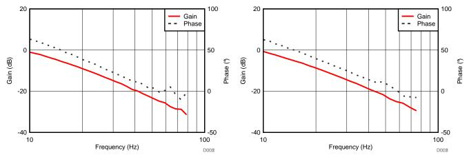
Figure 9. PFC Loop Gain/Phase at 300 W, 115 V
