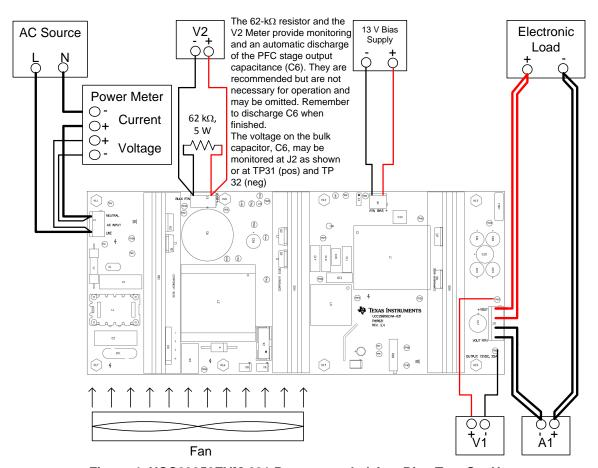
Figure 4. UCC29950EVM-631 Recommended Aux Bias Test Set Up
