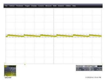
Figure 28. DC Coupled, V<sub>out</sub> 0 A, Aux Bias Burst is Approximately 8-ms Long, Burst Rep Interval is Approximately 340 ms
