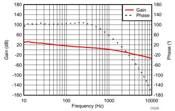
Figure 11. Gain/Phase vs. Frequency
