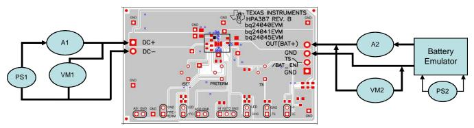
Figure 1. Original Test Setup
