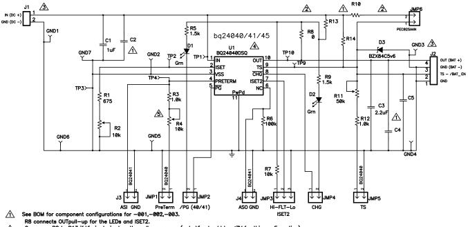
R8 connects OUTpull—up for the LEDs and ISET2.
