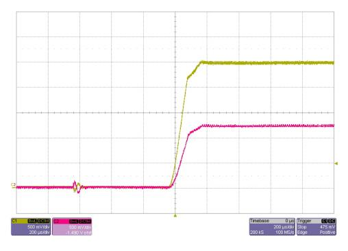
The photo below shows the 2.5V and 1.25V output voltage startup waveforms after the application of 12Vdc in. The outputs was unloaded. (500mV/DIV, 200uS/DIV)
