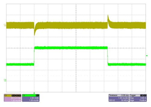
The photo below shows the 2.5V output voltage when the load current is stepped between 0.1A and 6A. Vin = 12Vdc. (50mV/DIV, 2A/DIV, 1mS/DIV)
