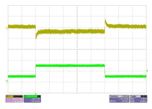
The photo below shows the 2.5V output voltage when the 1.25V load current is stepped between 1A and 3A. Vin = 12Vdc. (50mV/DIV, 2A/DIV, 1mS/DIV)
