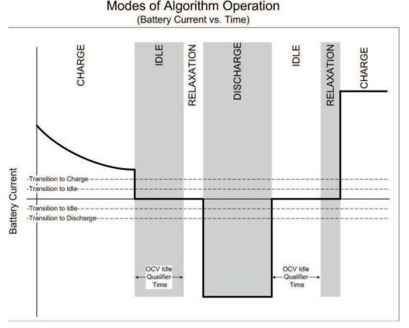
Figure 10-1. Gas Gauge Algorithm Modes of Operation
