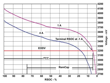
Figure 10-3. Discharge Simulation at 25 °C and 1 and 4 Amps Discharge Curves
