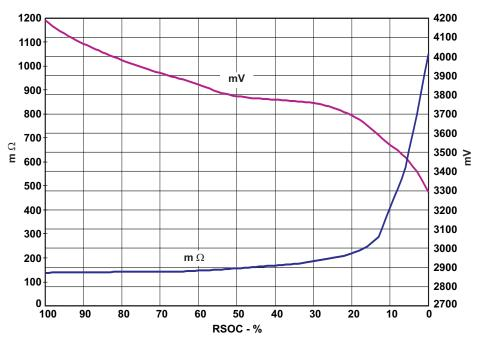
Figure 10-4. OCV and Impedance at 0°C
