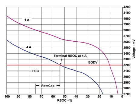
Figure 10-5. Discharge Simulation at 0°C and – 1 and – 4 Amps Discharge
