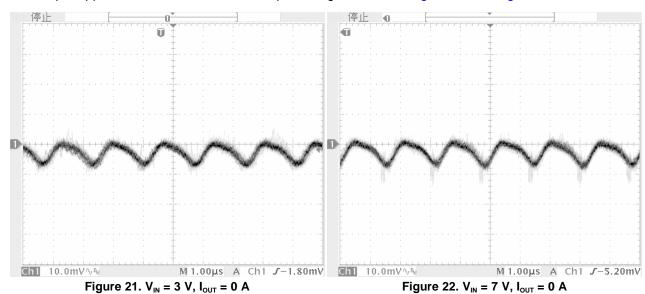
The output ripple waveforms with a 0.6-V output voltage is show in Figure 21 and Figure 22.
