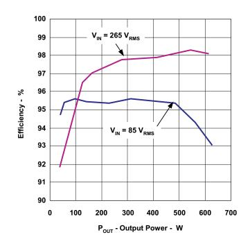
Figure 3. Efficiency at 85 VRMS and 265 VRMS
