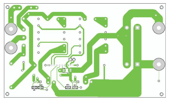
Figure 18. PR735 Power Stage Bottom Layer Layout (viewed from top)
