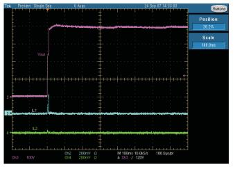
Figure 13. PR735 Start-Up at V<sub>IN</sub> = 265 VRMS,  $P_{OUT} = 0$  W
