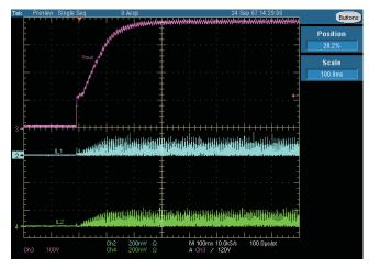
Figure 12. PR735 Start-Up at V<sub>IN</sub> = 85 VRMS,  $P_{OUT}$  = 600 W
