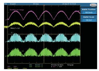
Figure 10. PR735 Inductor and Input Ripple Current at 85-VRMS Input, P<sub>OUT</sub> = 300 W
