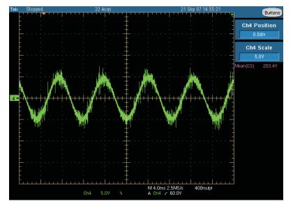
Figure 5. PR735 Output Voltage Ripple (5 V/DIV, ac coupled)
