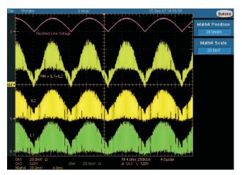
Figure 11. PR735 Inductor and Input Ripple Current at 265-VRMS Input, P<sub>OUT</sub> = 600 W
