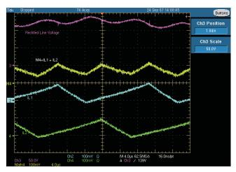
Figure 6. PR735 Inductor and Input Ripple Current at 85-VRMS Input at Peak Line Voltage
