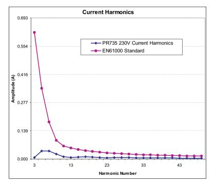
Figure 4. PR735 Current Harmonics with 230-VRMS Input
