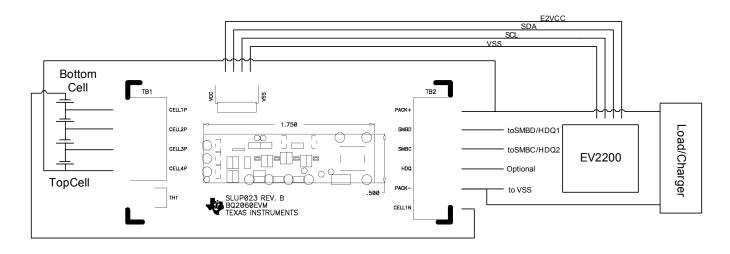
Figure 5-2. Circuit Module Connection to NiMH Cells and System Load/Charger
