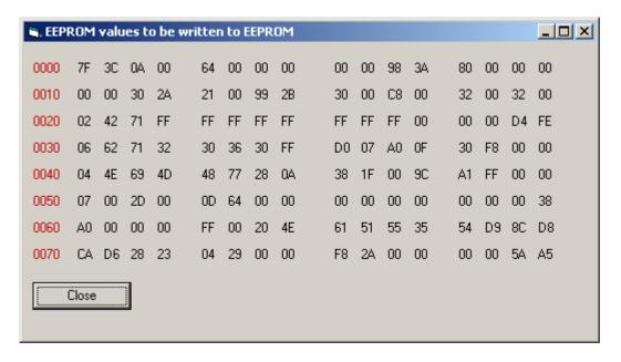
All data required for calibration is also held in the EEPROM for the bq2060, as highlighted in the following figure.
