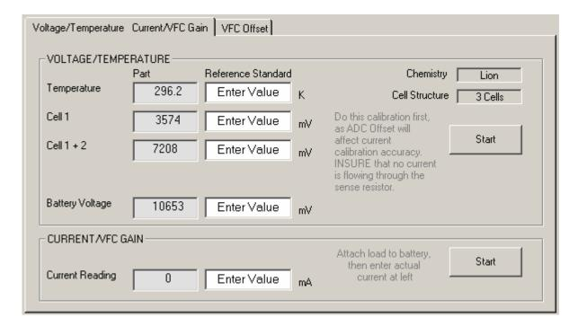
The Li-lon Calibration screen differs from the NiMH calibration screen by the individual cell voltages and cell structure. If the Chemistry or Cell Structure fields do not show the proper configuration in their respective fields, then select the bq2060 Data Screen Tab, select | Options | Initialize Device |, wait 5 seconds and then Return to the Calibration Tab.
