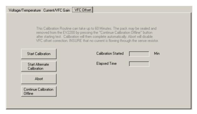
Default VFC Offset: To select this offset method click on | Start Calibration |. This method will apply an internal short (inside the bq2060) across the sense resistor. With the sense resistor shorted inside the bq2060 there is less chance that an external current can cause a poor offset calculation. This method does not compensate for slight offsets induced by the circuit board.
