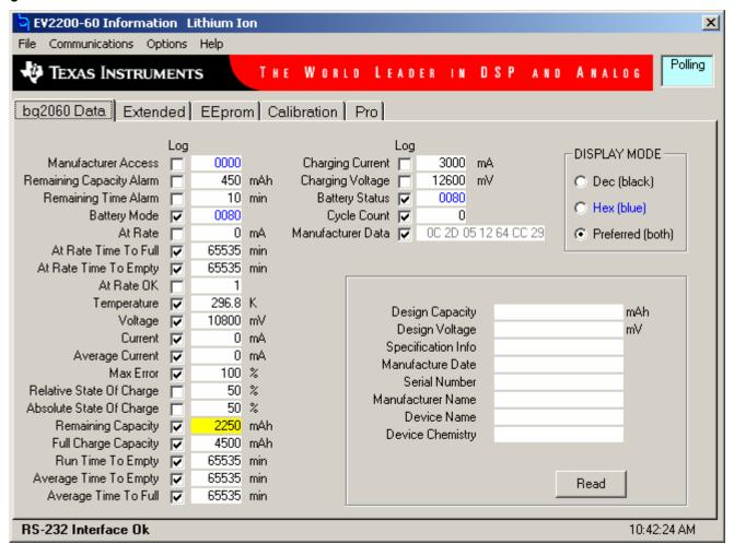
This SBS data screen shows the SBS data set, along with additional Static data shown in a box at the bottom right. By clicking on the 'Read...' button, the screen changes to show the static data from the bq2060.
