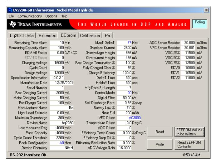
To read all the data from the bq2060 EEPROM, click on | Read |. To write to a selected location click on the desired location, type in the desired data, and hit the ENTER key. After a moment the next location will be highlighted. The entire EEPROM can be written this way.
