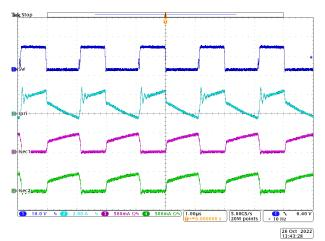
Figure 4-1. Steady State Waveforms ( $V_{IN}$  = 10 V, I<sub>OUT1</sub> = 1 A, I<sub>OUT2</sub> = 0.2 A, and I<sub>OUT3</sub> = 0.2 A)
