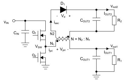
Figure 2-1. Isolated Buck Converter With Two Outputs
