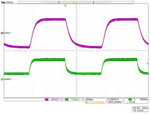
Figure 4-4. Load Step Response 50 mA to 200 mA ( $V_{IN}$  = 10 V,  $I_{OUT1}$  = 0 A, and  $I_{OUT3}$  = 0 A)
