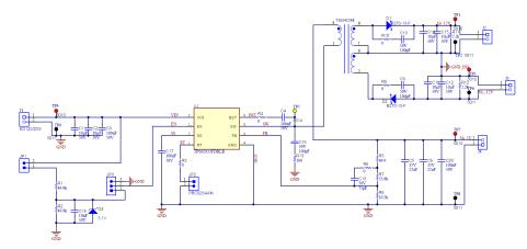
Figure 3-1. TPS62933F Two Output Isolated Buck Solution
