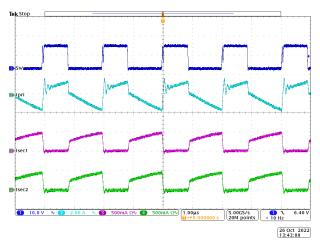
Figure 4-2. Steady State Waveforms ( $V_{IN}$  = 10 V, I<sub>OUT1</sub> = 0 A, I<sub>OUT2</sub> = 0.2 A, and I<sub>OUT3</sub> = 0.2 A)
