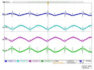
Figure 4-3. Ripple Voltage Waveforms (V<sub>IN</sub> = 10 V,  $I_{OUT1} = 1 \text{ A}$ ,  $I_{OUT2} = 0.2 \text{ A}$ , and  $I_{OUT3} = 0.2 \text{ A}$ )
