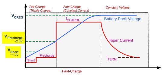
Figure 4-1. LiFePO4 Charge Profile
