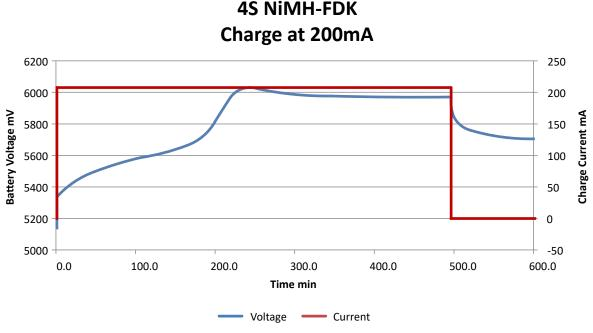
Figure 7-1. BQ25171 NiMH Charge Profile with 4 S FDK HR-AAULT Cells. 8 hr Timed Charge at 200 mA
