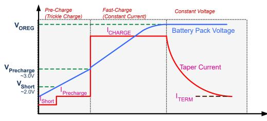
Figure 2-1. Typical Li-Ion Battery Charging Profile CC-CV
