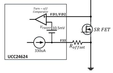
Figure 1-2. Adjustable Turn-off Threshold
