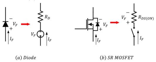
Figure 1-1. Equivalent Circuits for Diode and SR MOSFET
