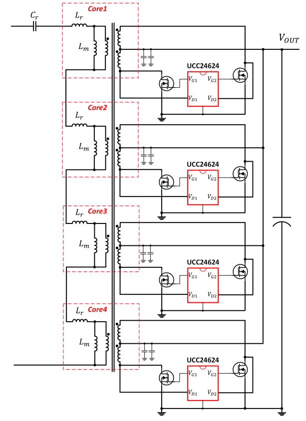
Figure 2-4. Multi UCC24624 with Matrix Transformer Application Schematic
