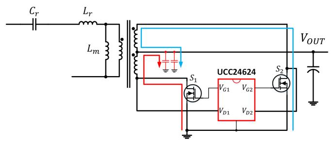
Figure 2-5. Recommended AC Coupling Ceramic Capacitors
