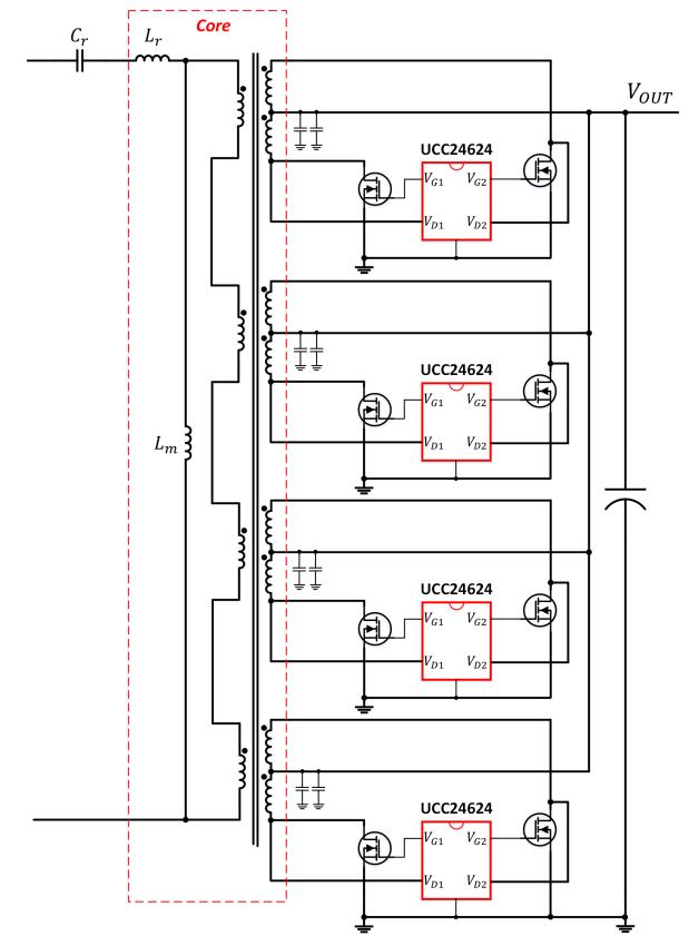
Figure 2-6. Multi UCC24624 with Novel Matrix Transformer Application Schematic
