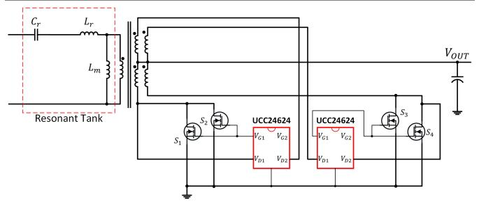
Figure 2-3. Dual UCC24624 Application Schematic
