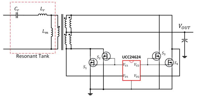
Figure 2-2. Single UCC24624 with Parallel MOSFETs Application Schematic
