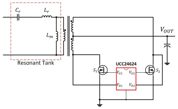
Figure 2-1. UCC24624 Typical Application Schematic
