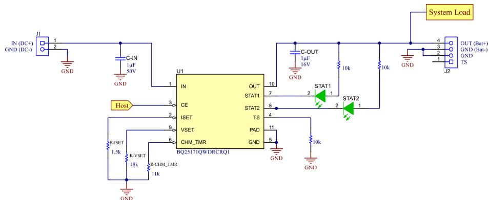
Figure 4-1. NiMH 200-mA Time Charge Design
