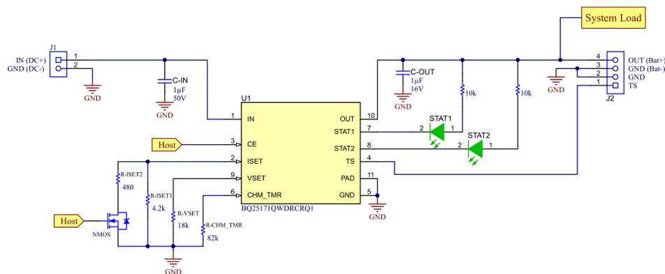
**Figure 3-1. BQ25171-Q1 700-mA/70-mA Fast Charge**
