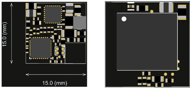
Figure 7. Layout Example – Double Sided
