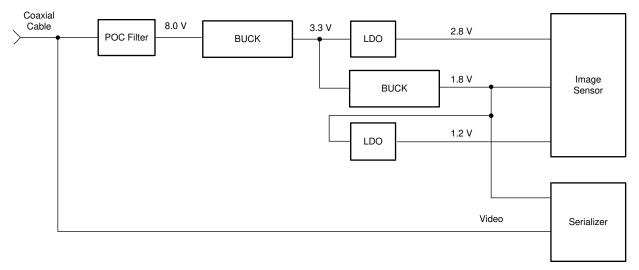
Figure 6. 1 MV + 1 LV + 2 LDO Configuration
