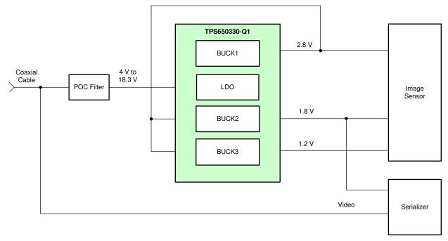
Figure 9. Using a DCDC Converter to Power the Analog Rail.
