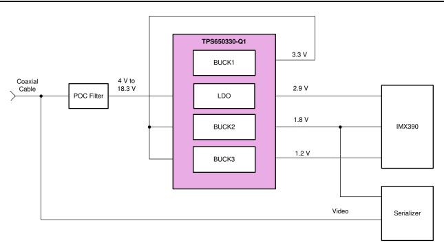
Figure 1. Sony<sup>®</sup> IMX390<sup>™</sup> Powered by the TPS650330-Q1 Power Management IC (Texas Instruments Reference Design TIDA-020003)
