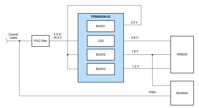
Figure 2. Aptina<sup>®</sup> AR02333<sup>™</sup> Powered by the TPS650330-Q1 Power Management IC (Texas Instruments Reference Design TIDA-050035)
