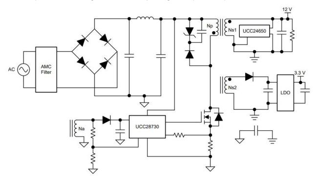
Figure 3. Block Diagram of TIDA-01560
