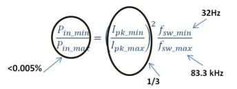
Equation 7 and Equation 8 estimate the standby power consumption by looking at the ratio of the min to max input power for the UCC28730 controller.
