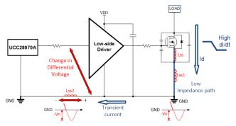
Figure 1. Simplified Schematic of a Low-side Gate Drive Using UCC27511A
