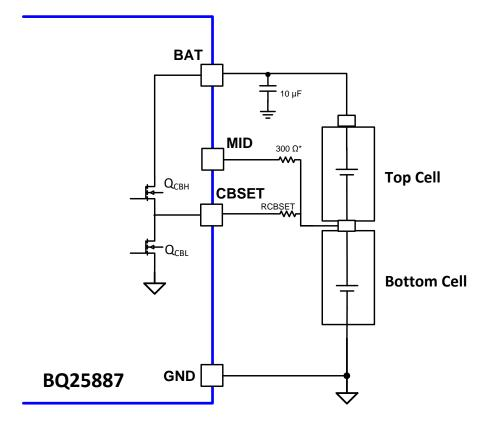
\*Note: The 300-Ω resistor on the MID pin is used to limit the current in cases where the bottom cell is plugged in reversely
