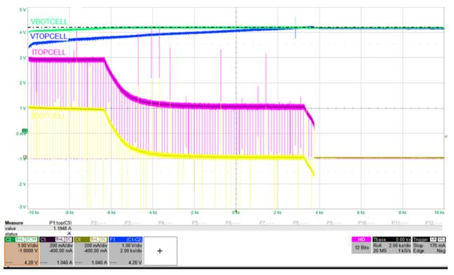
Figure 4. Charge Cycle with the Bottom Cell Voltage Higher Than the Top Cell Voltage
