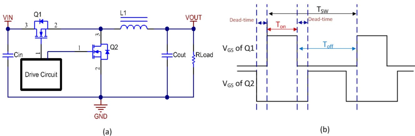
**Figure 2. Synchronous Buck Circuit, Drive Signal with Dead-time**
