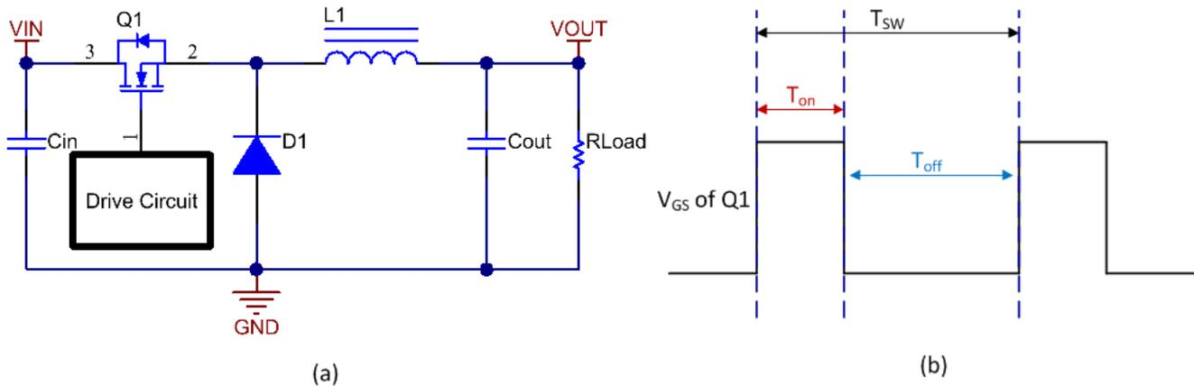
**Figure 1. Non-Synchronous Buck Circuit and Drive Signal**
