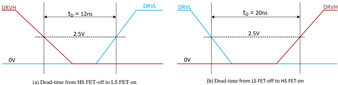
**Figure 4. Dead-time at ATE Test**
