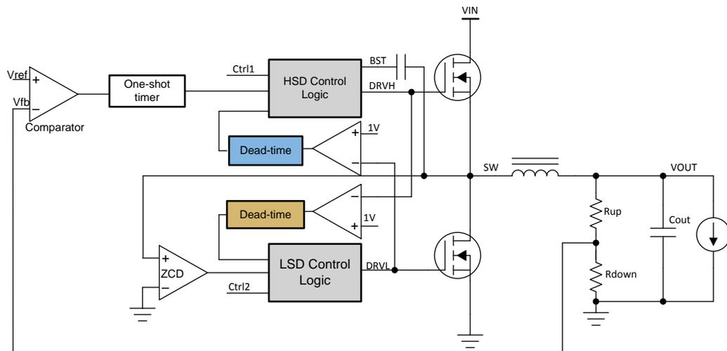
Figure 5. Block Diagram of the Dead-Time Control Circuit
