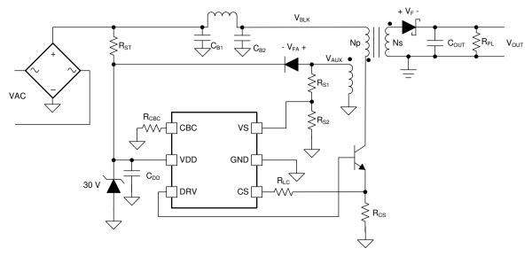
Figure 1. Simplified Application Circuit
