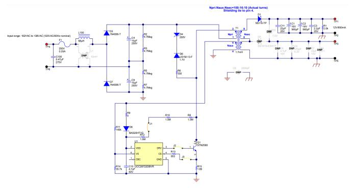
Figure 2. PMP21022 Schematic
