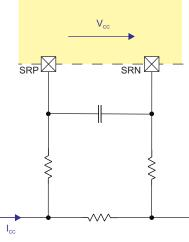
Figure 5. Current Calibration
