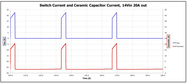
Switch and Input Ceramic Capacitor Currents at 14Vin and 20A Out
