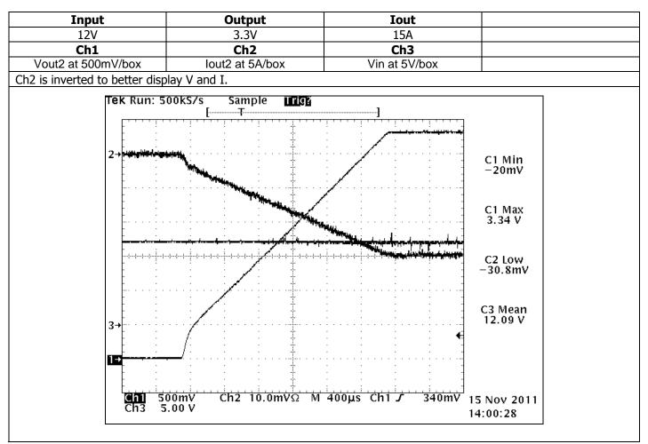
Measured Startup Waveform
