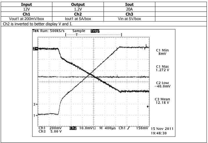
Measured Startup Waveform
