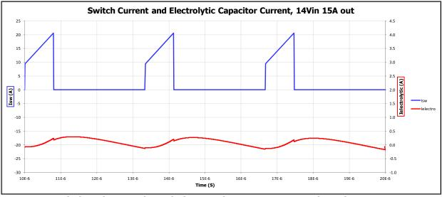
Switch and Input Electrolytic Capacitor Currents at 14Vin and 15A Out
