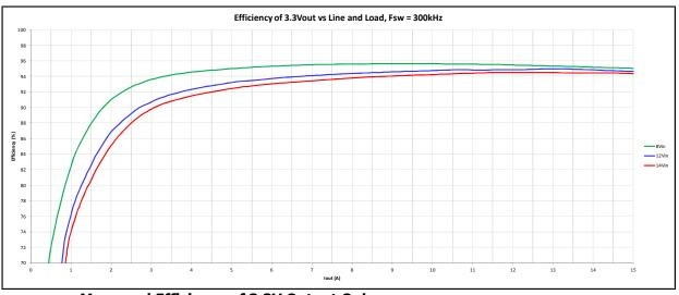
Measured Efficiency of 3.3V Output Only
