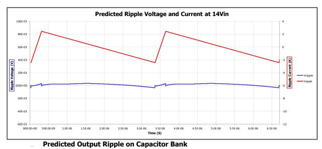
Neglecting any additional noise due to non-ideal layout, these results meet both the minimum capacitance
