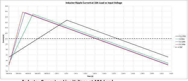
Inductor Current vs Line Voltage at 10A Load
