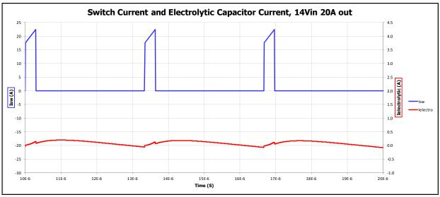
Switch and Input Electrolytic Capacitor Currents at 14Vin and 20A Out
