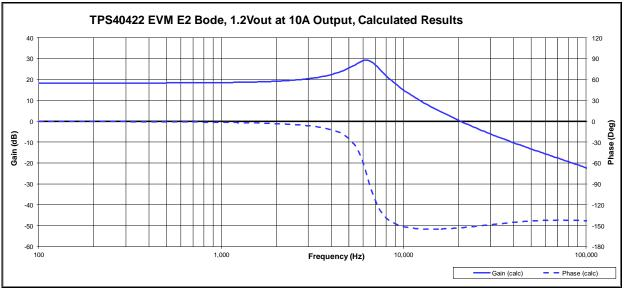
Calculated Plant Bode for 1.2V Output
