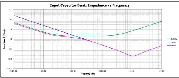
Input Capacitor Bank Impedance vs Frequency
