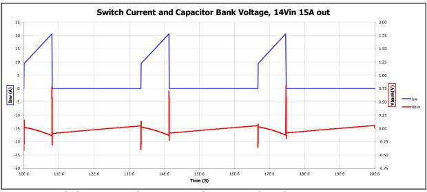
Switch Current and Input Bus Voltage at 14Vin and 15A Out
