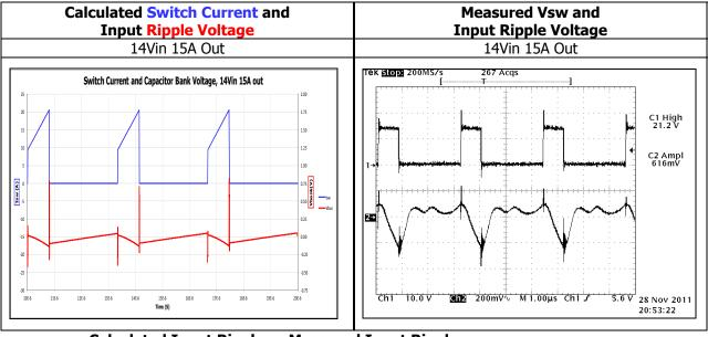
Calculated Input Ripple vs Measured Input Ripple
