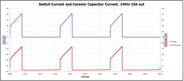
Switch and Input Ceramic Capacitor Currents at 14Vin and 15A Out
