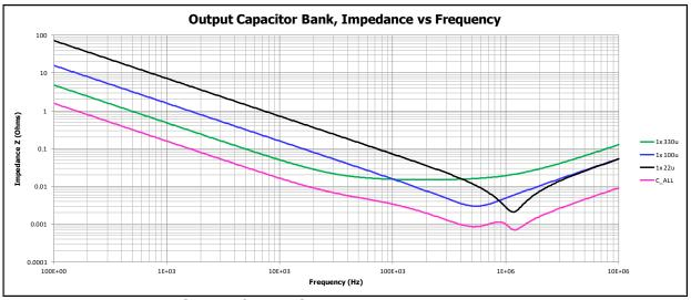
Output Capacitor Bank Impedance vs Frequency
