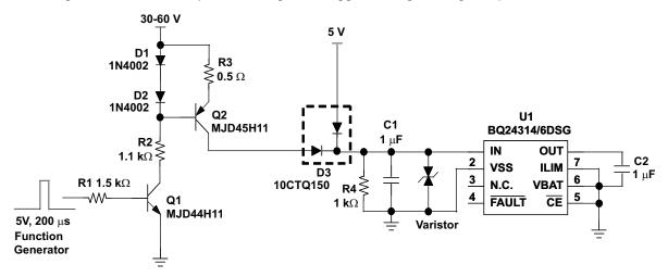
Figure 1. High-Voltage Pulse Transient Test Schematic
