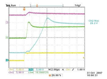
Figure 6. Vin From 5 V to 45 V, 2- $\mu s$  Time Scale Zoom in Detail, CH2 5 V/div
