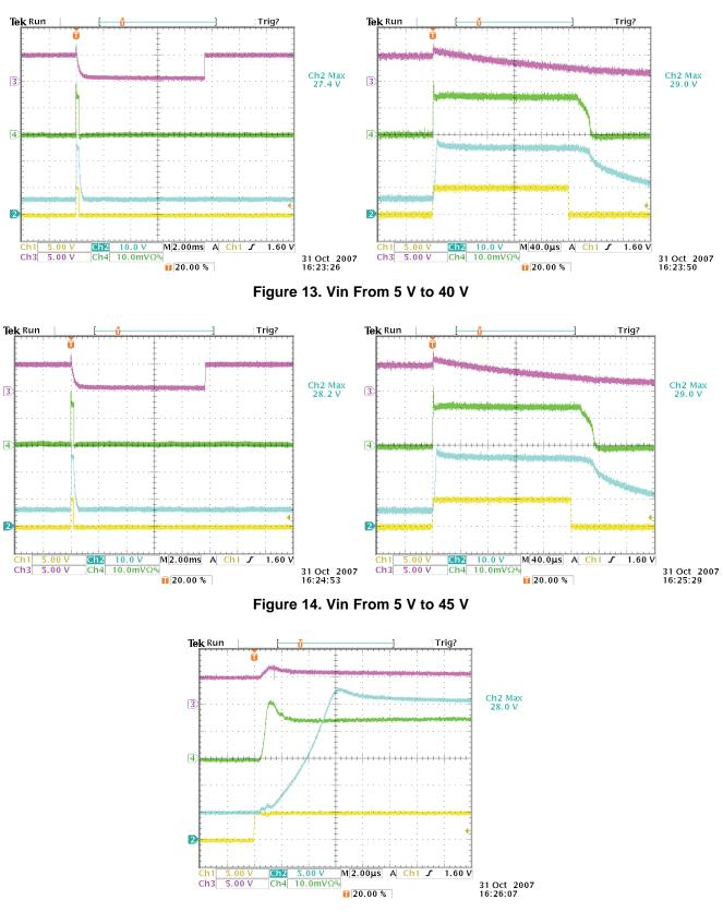
Figure 15. Vin From 5 V to 45 V, 2- $\!\mu s$  Time Scale Zoom in Detail, CH2 5 V/div
