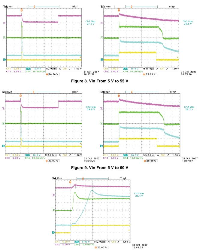
Figure 10. Vin From 5 V to 60 V, 2- $\mu$ s Time Scale Zoom in Detail, CH2 5 V/div
