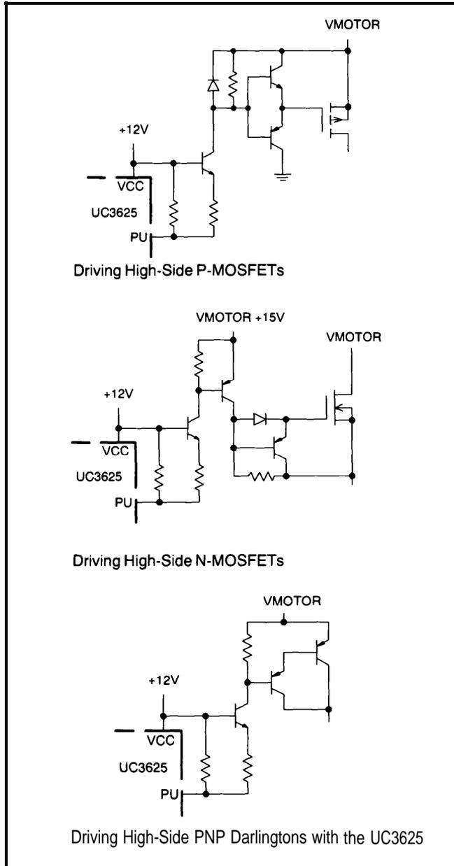
Although capable of 50mA current sinking, the open collector outputs are normally operated with lower currents to minimize the power supplied by the high-voltage supply.
