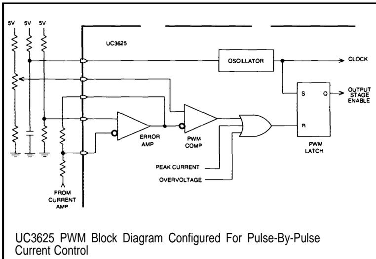
UC3625 PWM Block Diagram Configured For Pulse-By-Pulse Current Control
