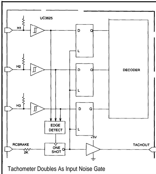
Tachometer Doubles As Input Noise Gate
