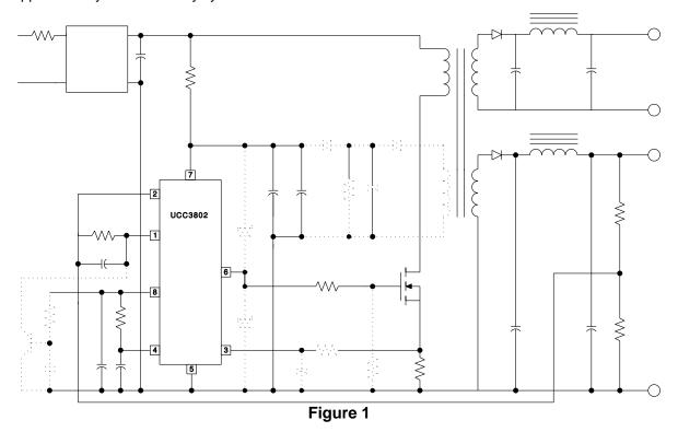
Figure 1 illustrates a nonisolated off-line flyback. Dotted components may be eliminated using the UCC3802 family.
