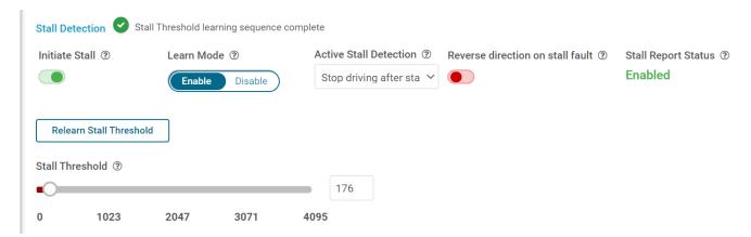
Figure 4-11. Stall detection configuration panel in Learn Mode
