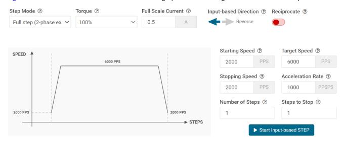
Figure 4-7. Settings and Controls of the Step Mode
