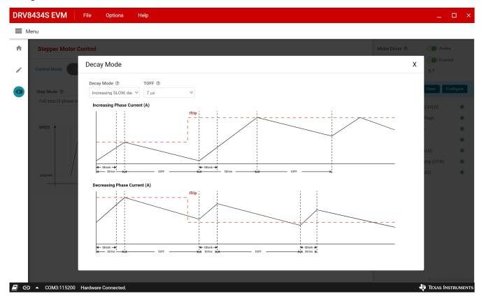
Figure 4-9. DRV8434S EVM GUI (Decay mode)
