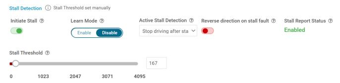
Figure 4-12. Stall detection configuration panel in Manual Mode
