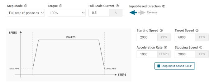
Figure 4-6. Settings and Controls of the Speed Mode
