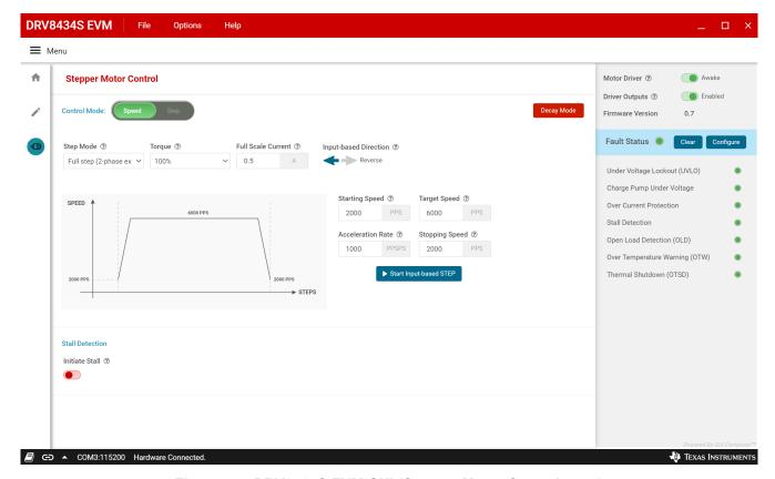
Figure 4-5. DRV8434S EVM GUI (Stepper Motor Control page)
