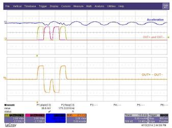
Figure 9. LRA Single-Cycle with Braking (Button 3)
