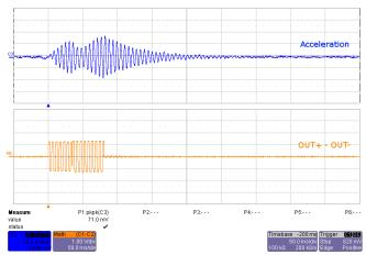
Figure 11. LRA Open-Loop Click Waveform (Button 4)
