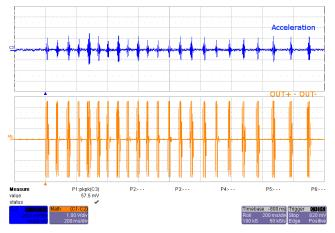
Figure 15. LRA Scroll Wheel Effect Waveform (Button 4)
