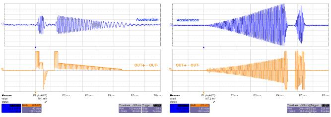
Figure 4. ERM Click and Bounce Waveform (Button 1)
