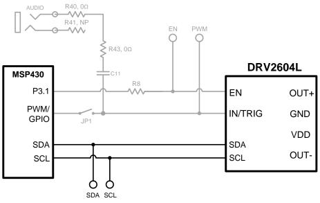
Figure 22. External I<sup>2</sup>C Input
