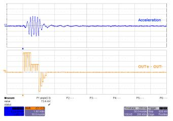
Figure 6. ERM Closed-Loop Click Waveform (Button 1)
