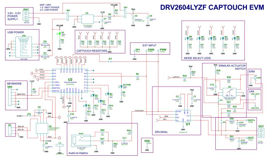
Figure 29. DRV2604LEVM-CT Schematic
