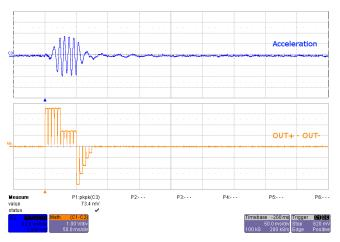
Figure 10. LRA Closed-Loop Click Waveform (Button 1)
