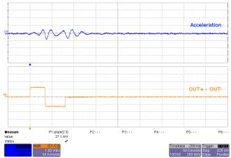
Figure 7. ERM Open-Loop Click Waveform (Button 4)
