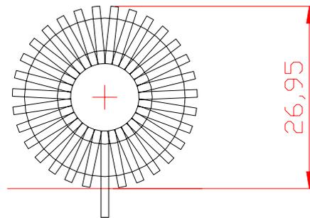
Lead length: 8mm-12mm, stripped and pre-tinned.
