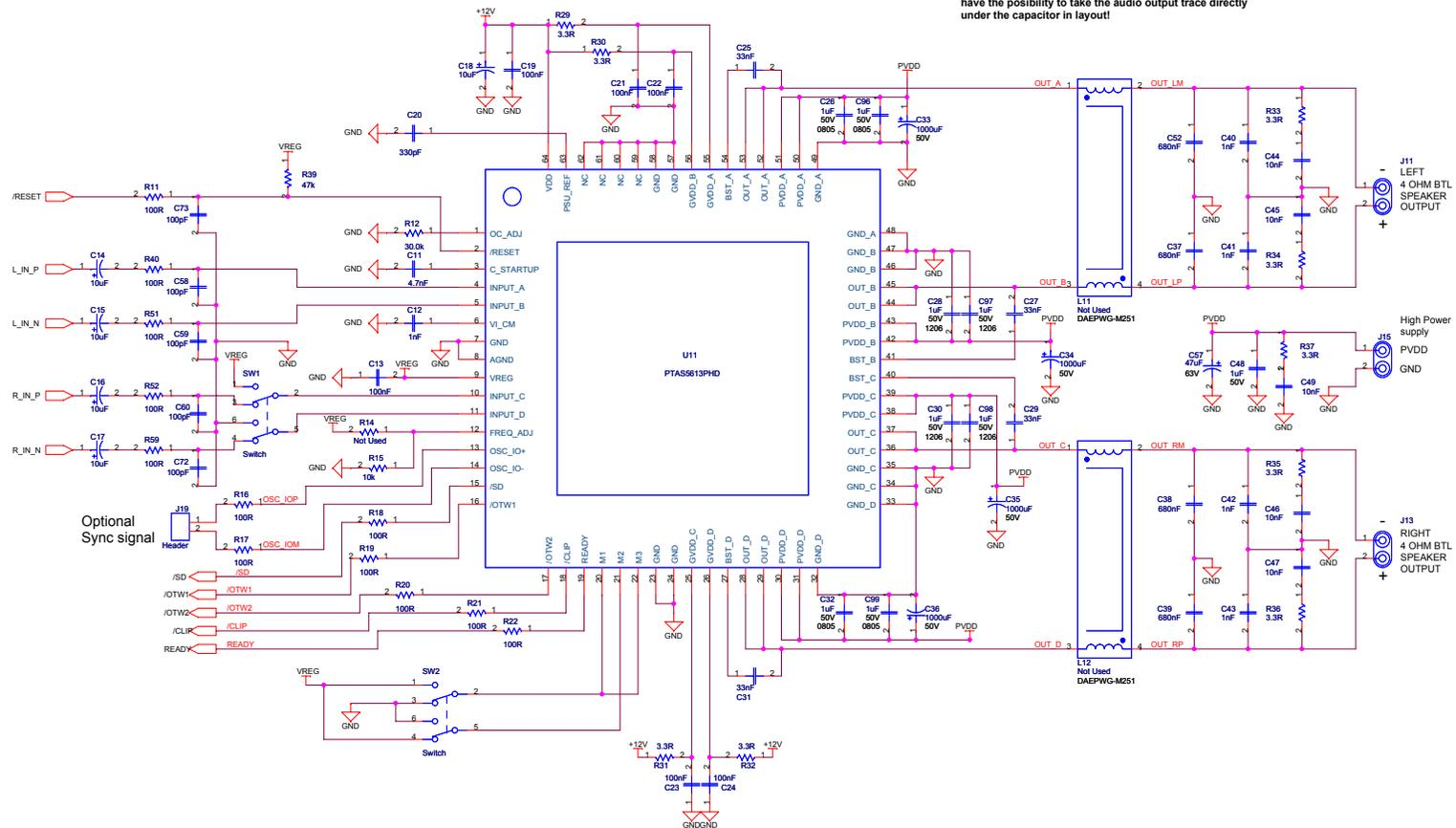
C28, C30, C97 and C98: It is important to choose either a 1206 or 1210 footprint for these decoupling capacitors to have the possibility to take the audio output trace directly under the capacitor in layout!
