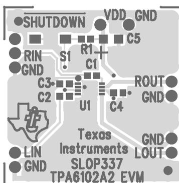
† Due to the very small size of the MSOP IC package, the standard part number TPA6102A2 is replaced with the code TIAJN.
