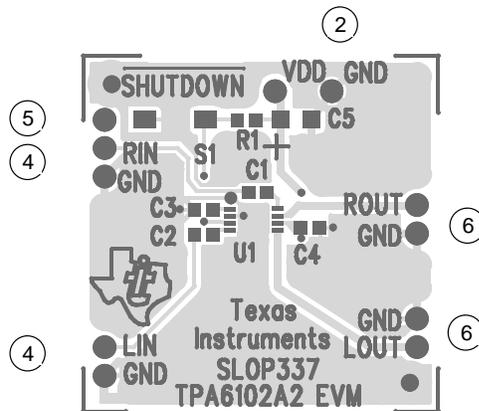
† Due to the very small size of the MSOP IC package, the standard part number TPA6102A2 is replaced with the code TIAJN.
