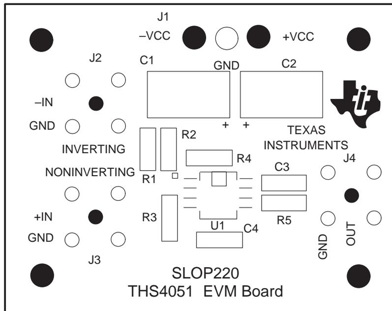
Figure 2–2. THS4051 EVM PC Board Layout – Component Side
