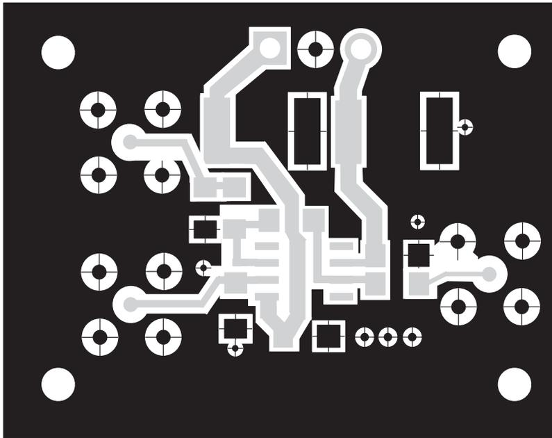
Figure 2–3. THS4051 EVM PC Board Layout – Back Side
