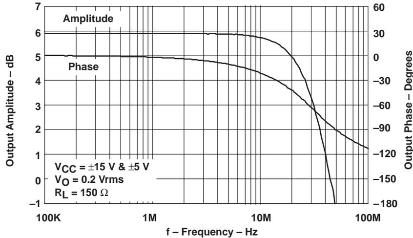
Figure 1–4 shows the typical frequency response of the THS4051 EVM using the inverting input ( $G = -1$ ). Typical  $-0.1$  dB bandwidths are 7 MHz and a  $-3$ -dB bandwidth of 30 MHz with a  $\pm 15$  V power supply. These bandwidths remain consistent when the power supply drops to  $\pm 5$  V.
