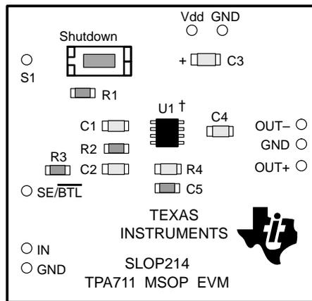
† Due to the very small size of the MSOP IC package, the standard part number TPA711 is replaced with the code TIABB
