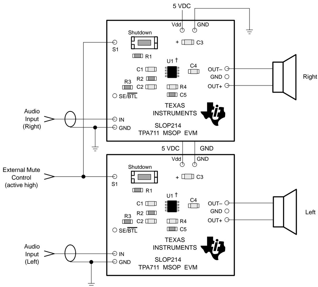
**Note:** The (SE/BTL) EVM pin is pulled to GND through a 20-kΩ resistor on the module.
