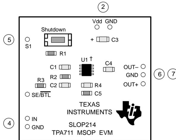
† Due to the very small size of the MSOP IC package, the standard part number TPA711 is replaced with the code TIABB
