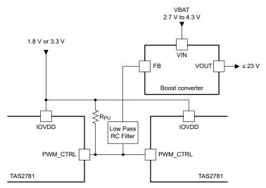
Figure 2-2. Multichannel Configuration Using PWM\_CTRL Pin With Open Drain
