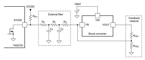
Figure 3-1. Hardware Connections
